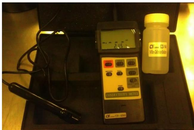
Figure 8: Electrical conductivity meter with calibration solution.
