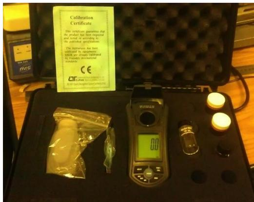
Figure 6: Turbidity meter and accessories: (left to right) Distilled water for cleaning, cleaning cloth, turbidity meter, testing vial, and calibration vials.
