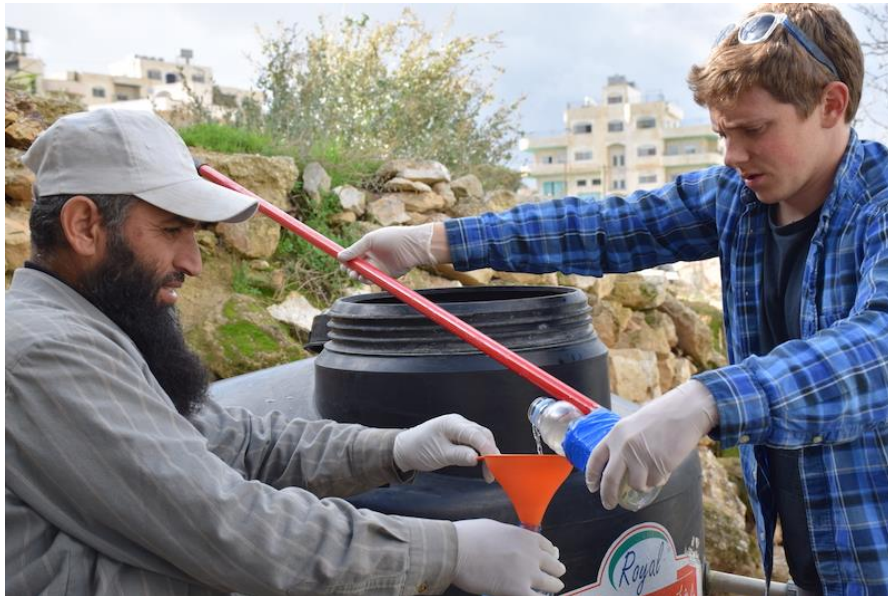
Figure 5: Grab sampling device being used to collect samples at Dar Salah. Photo credit: Antonia Bacigalupa Albaum
