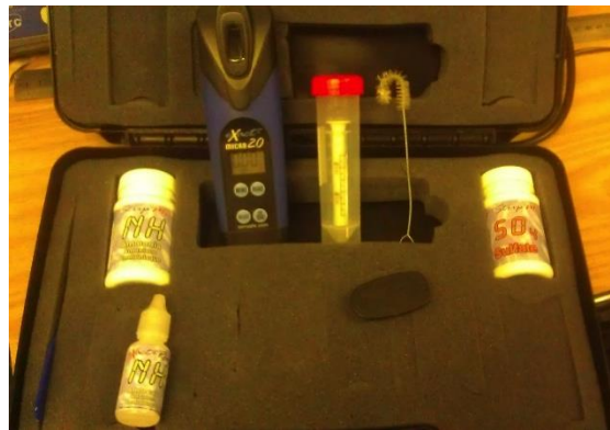
Figure 7: Photometer and accessories: (left to right): Ammonia testing reagents, photometer, dilution vessel and syringe, cleaning brush, photometer cover, and sulfate testing reagents.
