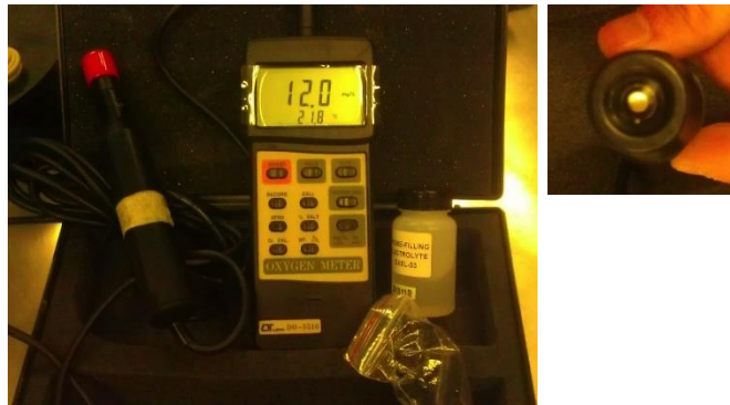
Figure 9: Dissolved oxygen meter and accessories: Left: (left to right): DO probe with protective cover, DO meter, extra electrolyte for refilling probe, and spare tips for DO probe. Right: head-on view of DO probe tip without protective cover.
