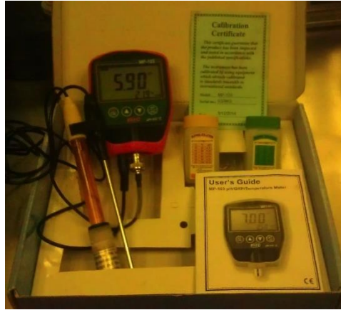
Figure 10: pH meter and accessories: (left to right) pH probe in 3 M KCl storage solution, temperature probe, pH meter, and calibration solutions.
