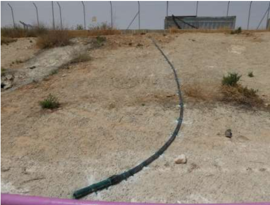
Figure 4: The sensor passes through a pipe located adjacent to the infrastructure of the channel.
